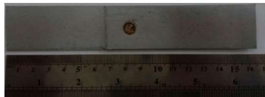
Figure 3. Resistance spot welded sample image
