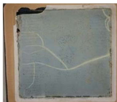
Figure 2. The anode layer of SOFC after experimental study.
