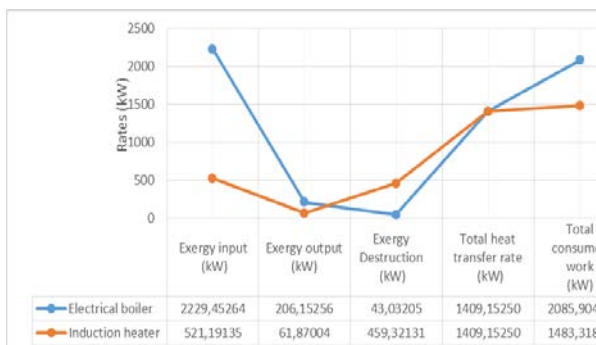
Figure 3. Energy and exergy rates in pasteurization systems with electric boiler and induction heater
