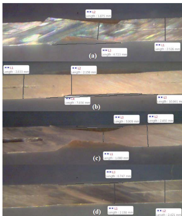
Figure 6. Macrostructures obtained at different electrode tip types and 5 kA welding current a) flat conical b) conical R3 c) conical round d) flat R6
