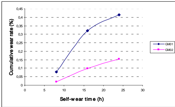
Fig 5. Cumulative wear curves of beads in vertical stirred mill.
