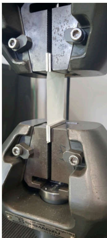
Figure 1. Tensile test specimen on the test machine.
