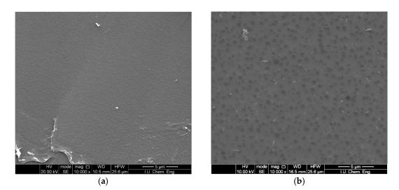
Figure 2. SEM images of membranes (5000×) (a) PAN 1; (b) PAN 2.
