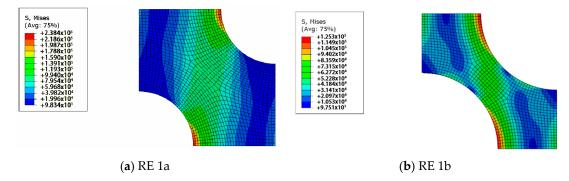
Figure 11. The von Mises stress distributions of RE 1.
