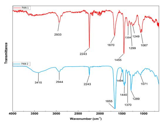
Figure 4. Results of FTIR analysis of PAN 1 and PAN 2 membranes.
