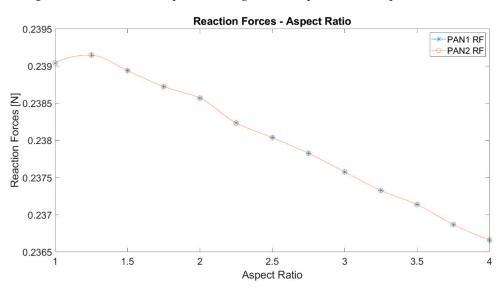
Figure 10. The total reaction force of elliptical membranes against the aspect ratio.
