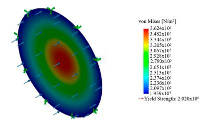
Figure 5. Equivalent stress distribution in a circular membrane.
