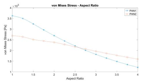
Figure 7. The maximum von Mises equivalent stress against the aspect ratio of elliptic membranes.
