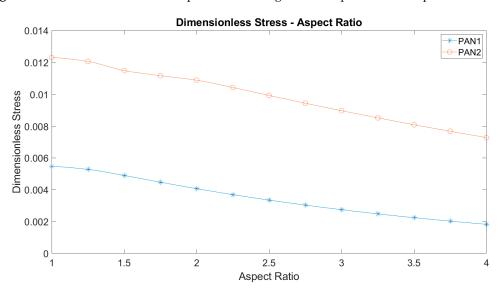
Figure 8. The maximum dimensionless stress against the aspect ratio of elliptic membranes.
