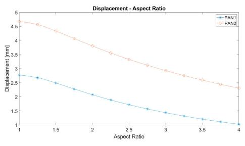
Figure 9. The maximum displacements against the aspect ratio of elliptic membranes.
