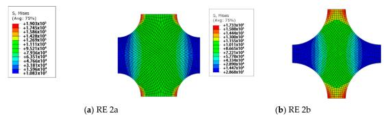
Figure 12. The von Mises stress distributions of RE 2.
