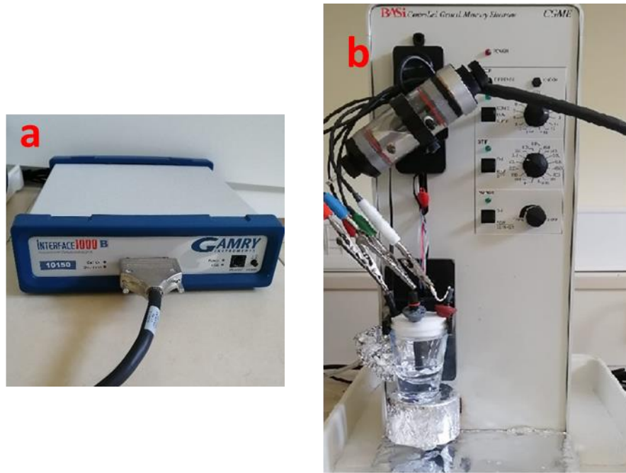
Şekil.4.1. a) Gamry Interface 1000B Potentiostat/Galvanostat/ZRA b) Bioanalytical System (BAS) C3 hücre sistemi
