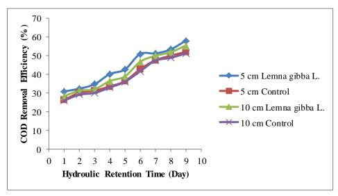
Fig 7. The COD removal efficiencies according to the various HRT and depths.
