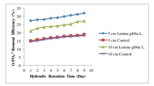
**Fig 6.** The O-PO<sub>4</sub><sup>-3</sup> removal efficiencies according to the various HRT and depths.
