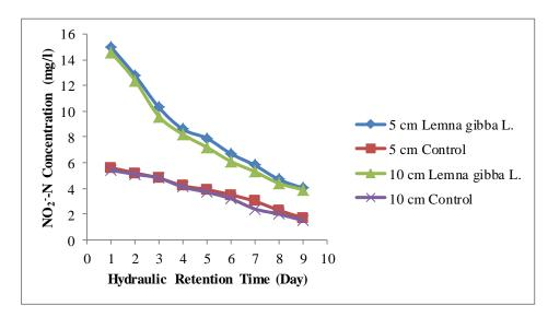
Fig 4. The  $NO_2^-$ -N concentrations according to the various HRT and depths.
