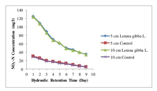
**Fig 5.** The  $NO_3$ -N concentrations according to the various HRT and depths.
