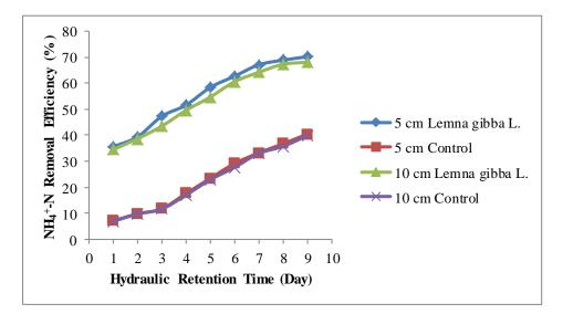
**Fig 3.** The NH<sub>4</sub><sup>+</sup>-N removal efficiencies according to the various HRT and depths.
