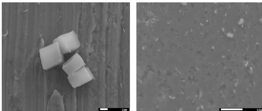
Figure 4. SEM pictures of MOF-5 and MOF-5/PI mixed matrix membrane
