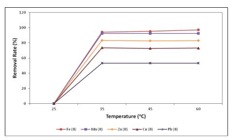
Figure 2. Effect of temperature on Fe(II), Mn(II), Zn(II), Cu(II) and Pb (II) ions adsorption by Şile-Kömürcüoda clay soil
