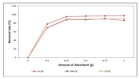
Figure 1. Effect of adsorbent amount on Fe(II), Mn(II) and Zn(II) ions adsorption by Sile-Kömürcüoda clay soil
