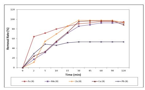
Figure 3. Effect of time on Fe(II), Mn(II), Zn(II), Cu(II) and Pb (II) ions adsorption by Şile-Kömürcüoda clay soil
