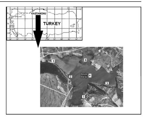
stations shown in Fig. 1 from Beyler reservoir. Ekman grab sampler was used to collect the reservoir bottom sediments. To avoid contamination, sediment was transferred into precleaned polythene bags and then frozen.
