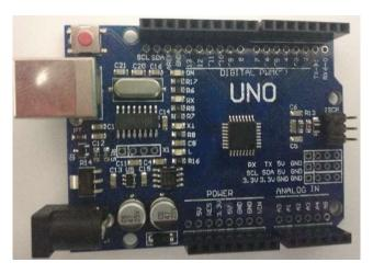
Figure 1 Arduino UNO microcontroller board
