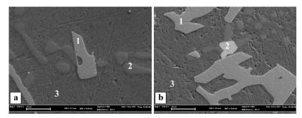
Figure 3. SEM images of LM6 alloys which were alloyed by 0.05% Zr (a) and 0.15% Zr.
