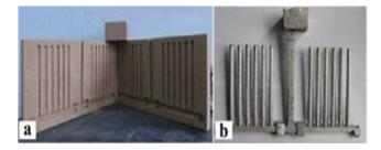
Figure 1. The image of sand molds (a) and image of casting parts (b)
